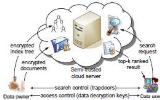
Fig. 1. The architecture of ranked search over encrypted cloud data
