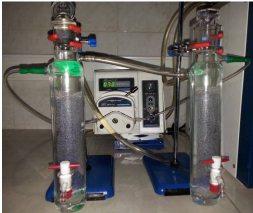
Fig. 1. Photograph of the running MDLM system for Pb(II) extraction.
