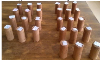
Figure 2.1: UCS samples with various percentages of flyash and lime
