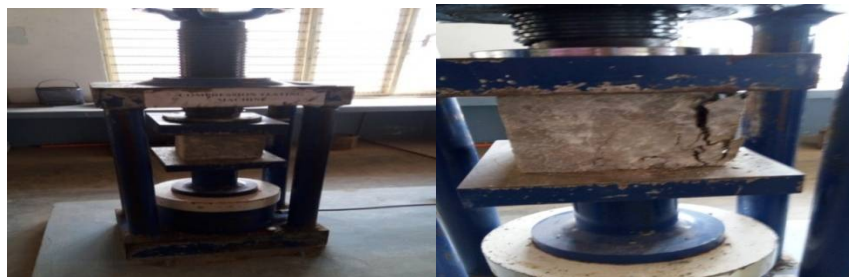
Fig 3 Compression testing of concrete cubes specimen
