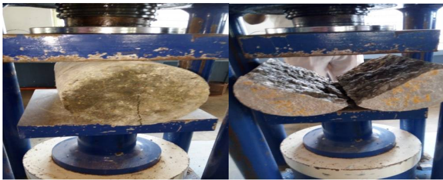
Fig 5 Split tensile testing of concrete cubes specimen
