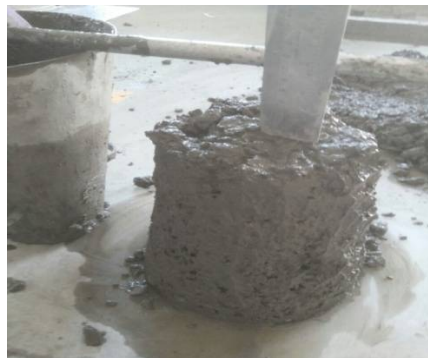
Fig 1 Slump cone test for M25 concrete
