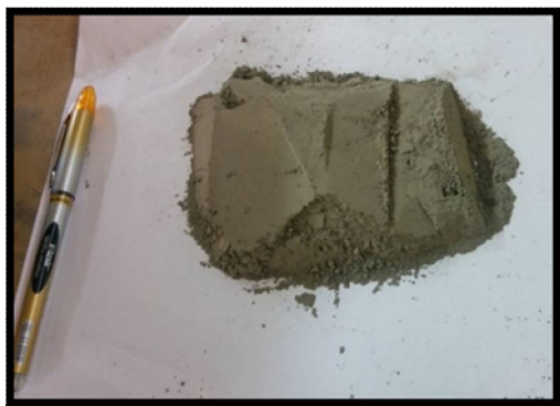
Figure 1: Paper Sludge Ash
