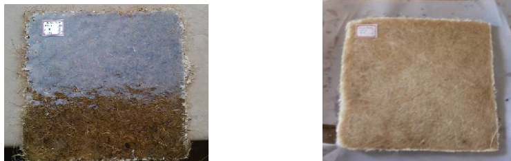
Figure 3: Coir and Sisal fibre composite panels of different thickness.
