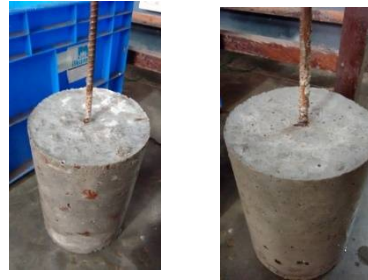
Figure 8 Sample without Calcium Nitrate and with Calcium Nitrate post accelerated corrosion test.
