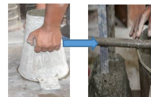
Figure 3 Slump cone test
