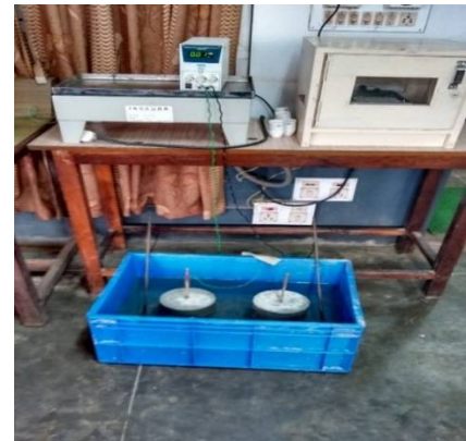
Figure 4 Set up of Accelerated Corrosion Test in the Physics Lab
