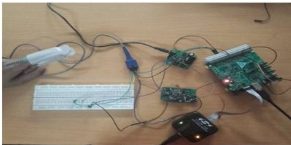
Figure 7: Experimental set-up showing connection of Debug adapter to Target board
