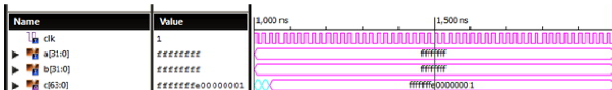
Figure 7: Simulation Result of 32x32 bit Vedic Multiplier
