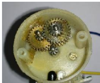
Figure 2: Positioning the IR transmitter and receiver into the primary shaft
