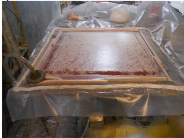
**Fig.4** Manufacture of Glass fibre laminate using Vacuum hand lay – up technique [5].
