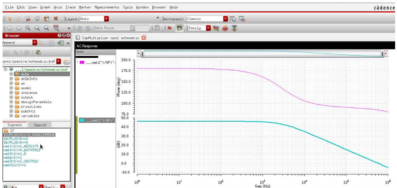
Fig. 6 Frequency Response of RC LPF showing Power Consumption in the Circuit.
