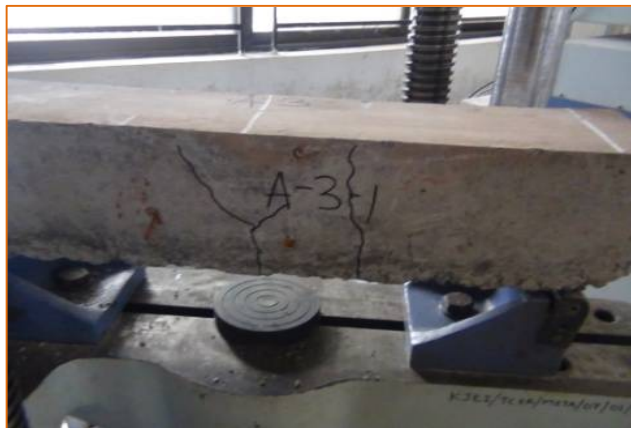
Fig. 5 Flexure and shear cracks for N beam
