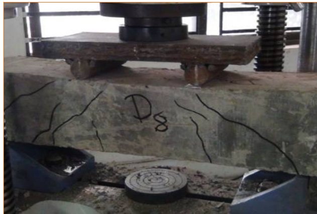
Fig. 5 Flexure and shear cracks for N beam
