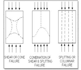
Fig..2 Failure Pattern of Specimen on Pervious Concrete Cubes
