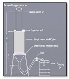
**Fig.7 Permeability Test Arrangement**
