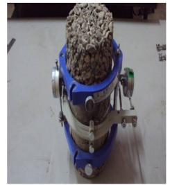
Figure8 Poisson's Ratio Test Arrangement
