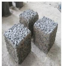
**Fig.9 Pervious Concrete**
