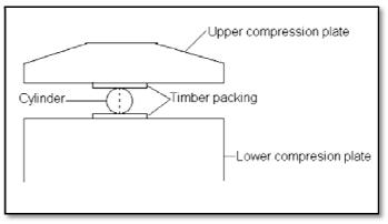
Fig. 3 Split Tensile Test on Pervious Concrete Cylinders
