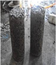
**Fig.11Pervious Concrete Cylinders**
