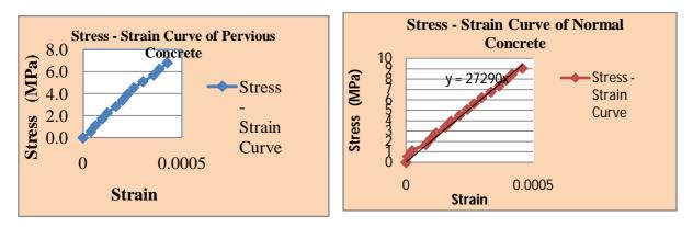
Fig. 4.5 (a) Young's Modulus for Pervious Concrete Fig. 4.5(b) Young's Modulus for Normal Concrete Specimen
