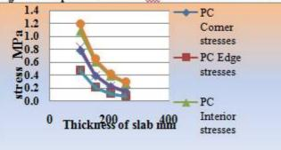
Fig. 4.7 Comparison of max +ye stress of PC and NC in X direction
