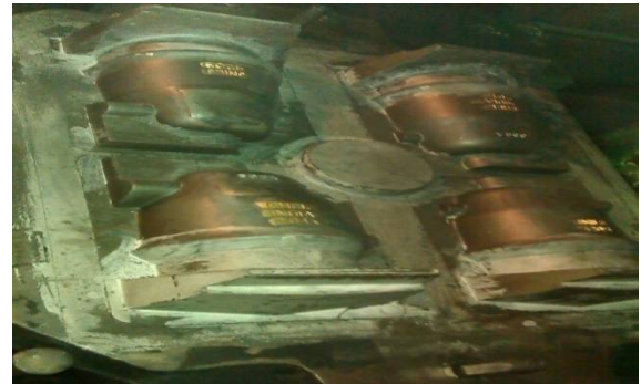
Fig.3:- Drag of Gating system of Socket cap 420 KN
