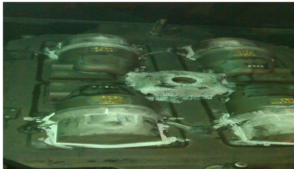
Fig. 2:- Cope of Gating system of Socket cap 420 KN
