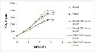
Fig 8. Variation of NOx with Brake Power
