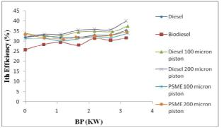
Fig 3. Variation of Indicated Thermal Efficiency with BrakePower
