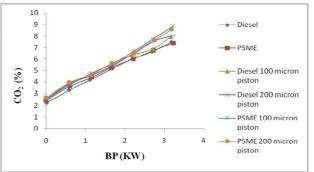
Fig 7. Variation of CO<sub>2</sub> with Brake Power
