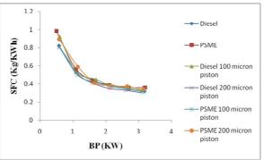
Fig 1. Variation of SFC with Brake Power
