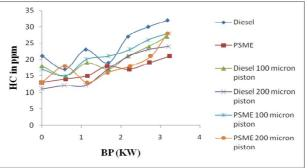
Fig 5. Variation of HC with Brake Power
