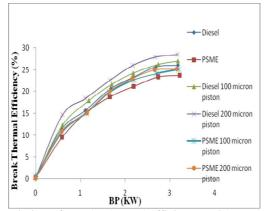
Fig 2. Variation of Break Thermal efficiency With Brake Power
