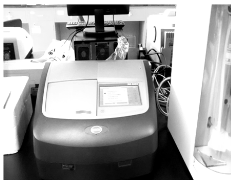
Plate (5) UV VIS Spectrophotometer with RFID Technology
