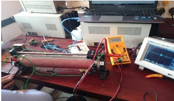
Fig. 8 Completed Laboratory Setup of the Bidirectional AC/DC Converter
