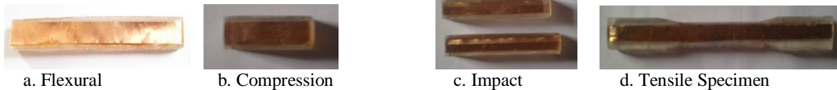
Fig. 2 Flat Specimens with Electrical Inserts before Testing
