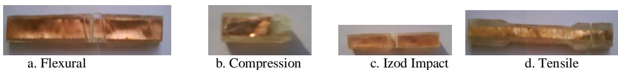
Fig. 3 Flat Specimens with Electrical Inserts after Testing
