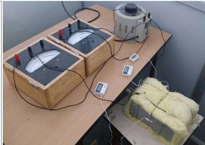
Fig 4: Thermal conductivity Test Setup
