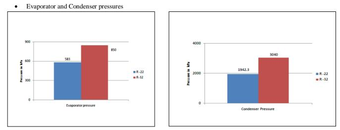
The operating pressures of R-32 are 45.78 % higher at evaporator and at condenser it is 56.5 % higher than that of R -22. As R-32 is an eco friendly refrigerant, it can be used in RAC systems, by altering the manufacturing process, so as to get sufficient strength to withstand high operating pressures.
