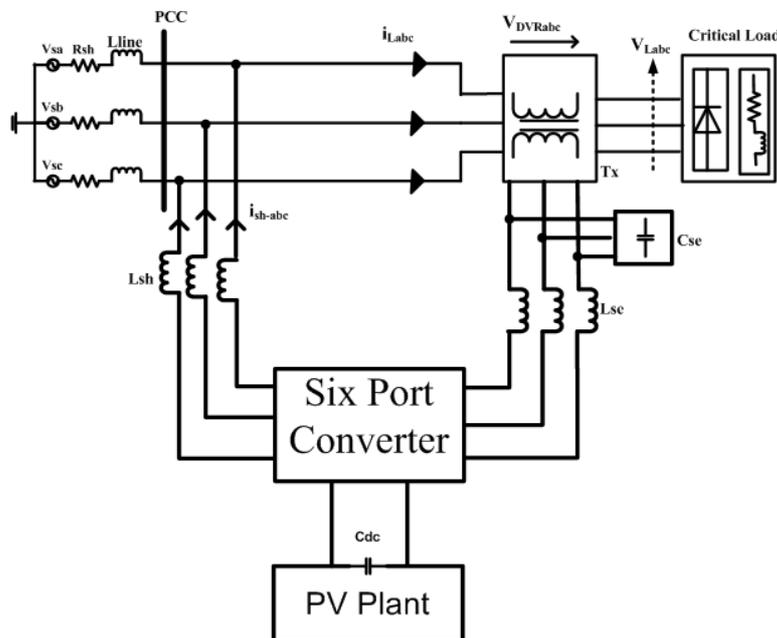
Fig.2. Proposed configuration of integrated PV and DVR systems
