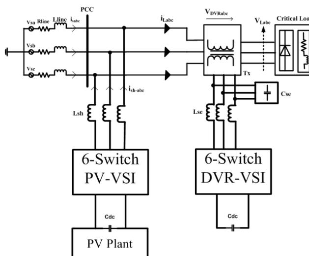
Fig.1 On-site PV generation and sensitive load protection using self-supported DVR system.
