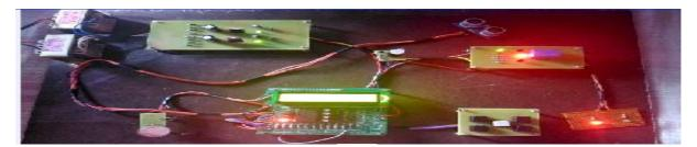
[3] When ultrasonic sensor detects any obstacle the alarm produces sound and the distance between the vehicle and the obstacle is displayed in the LCD display. This figure describes that the transmitter of ultrasonic sensor produces the waves simultaneously the time value starts counting in the controller and when the wave finds any obstacle it is reflected back and reaches to the receiver. And based on the time value the distance is calculated also will be displayed in the LCD display.
