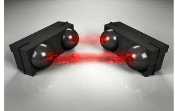
Intensity modulation with direct detection (IM/DD) is generally used in VLC systems. Many modulation techniques based on IM/DD have been proposed, including single-carrier modulation like on-off keying (OOK) or pulse position modulation (PPM) and multi-carrier modulation such as orthogonal frequency division multiplexing (OFDM) in
