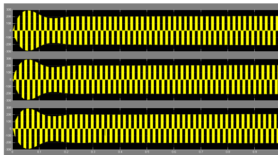
Fig. 9. Three phase output voltage wind speed = 10M/S (Without Converter)
