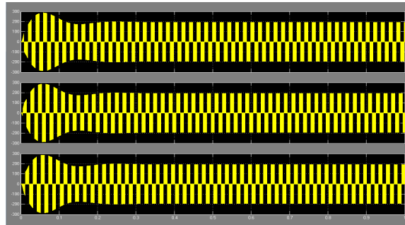
Fig. 8. Three phase output voltage wind speed = 7M/S (Without Converter)
