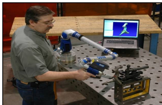
Fig-6 Actual Measurement Of Part Using Faro Arm
