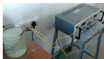
Fig 2.3 The DC power supply used in corrosion process
