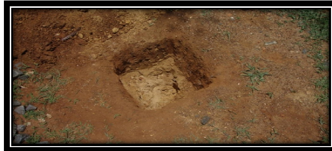
Fig.3. Pits for C.B.R tests. Generally pits are made to perform the C.B.R tests to know the inner bearing capacity of the soil.
