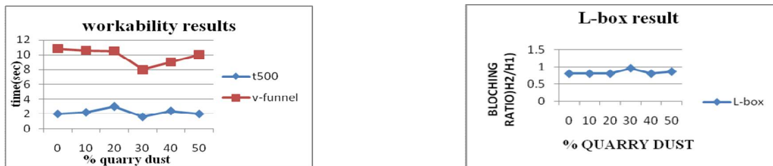
Fig.4. Graph representing flow ability results
