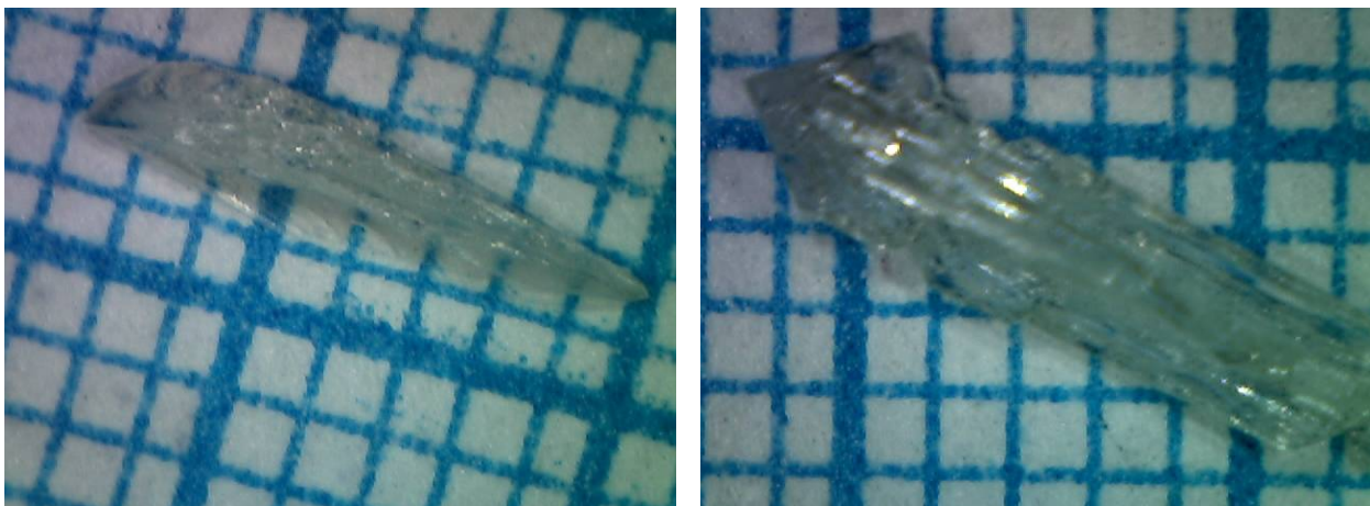
Fig. 1 Platelet type crystal Grown by \text{CaCl}_2 (Solution A) Fig. 2 Platelet type crystal Grown by \text{Ca}(\text{OH})_2 (Solution B)
