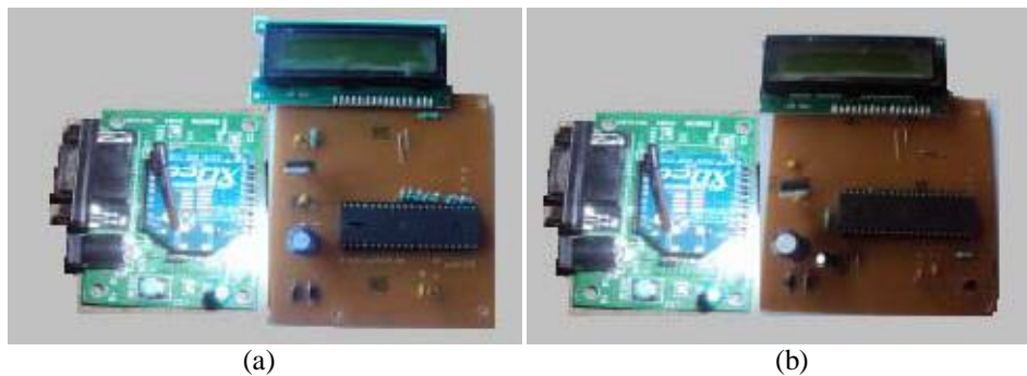
Fig. 3 Real Implemented System (a) Transmitter module with Zigbee base PCB (b) Receiver Module with Zigbee base PCB.
