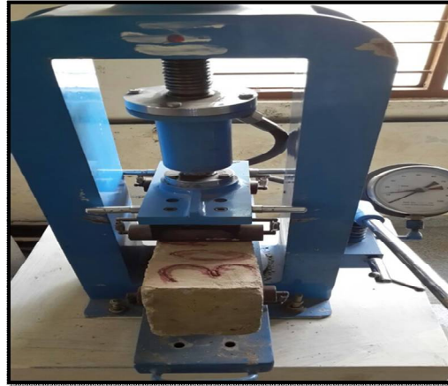
Fig 4.2: Flexural Test for Beam
