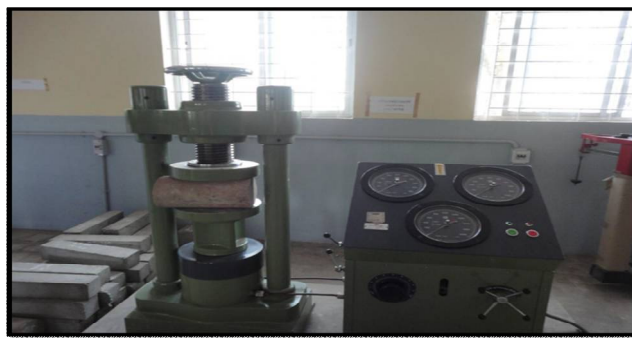
Fig 4.1: Split Tensile Test for cylinder
