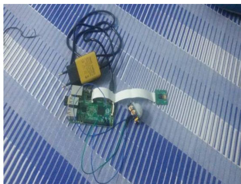
Fig3-Hardware setup of proposed system showing PIR sensor and Pi-camera with network adapter with Adapter and connecting wires.
