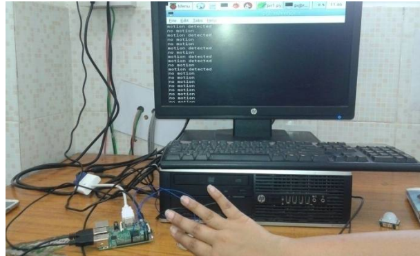
Fig 4-Screen showing motion detection by PIR sensor Whenever there is motion or movement Here, hand is used for detecting motion
