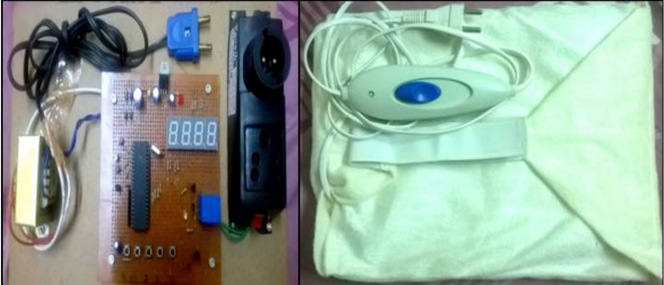
Fig 4: Hardware Model of Timer Based Electric Heating Pad
