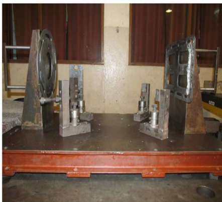
Figure 2: Adaptive averaging fixture for 6"/9" SM Pump Body
