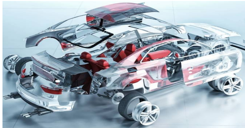
Fig 1: Car Body Frame Assembled explode view
