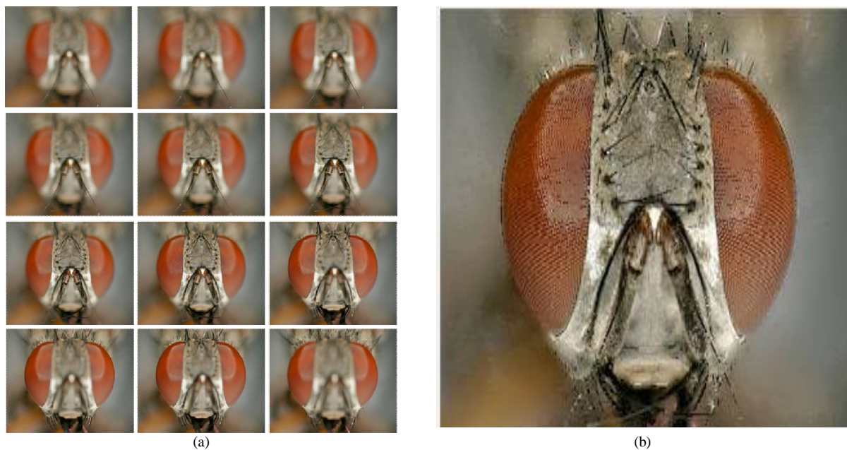
Figure 10 (a) Shows few partially focused image stack of fly eye taken from internet source. Figure 10 (b) Shows fully focused image of Fly eye (rough and irregular object)
