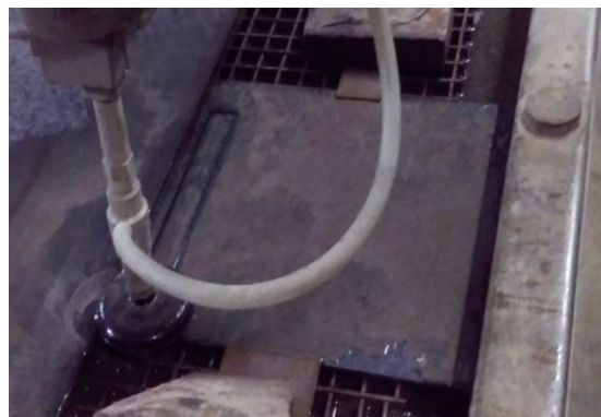
Fig 4. Laminated plate subjected to water jet cutting
