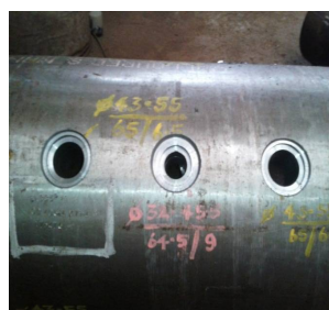
Figure 1(a) – Sequential drilling of holes carried out in the pipe 1(b) Preheating being carried out at 220^\circ\text{C} before the start of welding .
