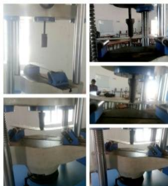
Fig.5 Bending test of specimen
