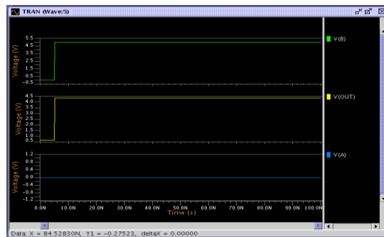
Fig.5 Simulation for Modified GDI XOR gate
