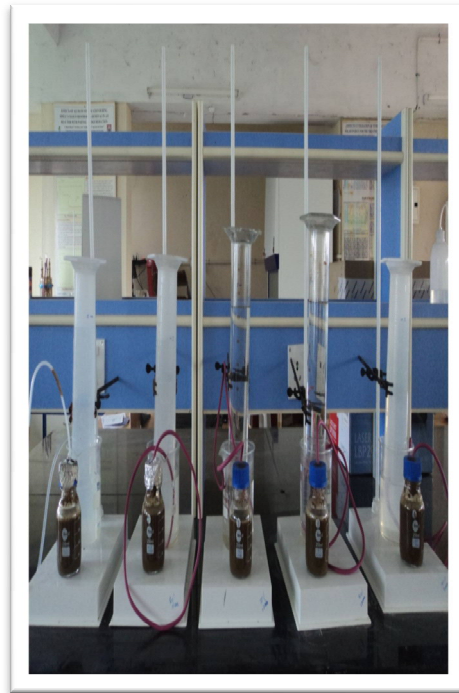
Fig 2.3 Experimental setup of anaerobic biodegradability assay
