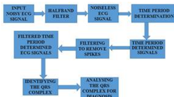
Fig. 2. Architecture diagram of the proposed ECG system
