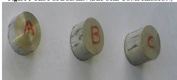
COLD UPSETTING TEST SPECIMEN BEFORE COMPRESSION WITH ASPECT RATIO (A) 0.5 (B)0.75 (C) 1.0
