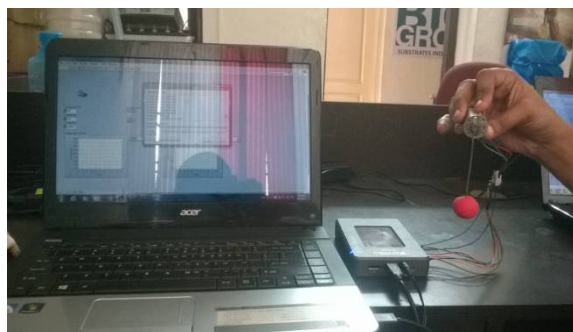
Figure.4 Experimental Setup of Inverted Pendulum System
