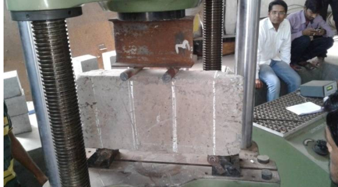
Figure 2 Beam Specimen and Experimental Set Up
