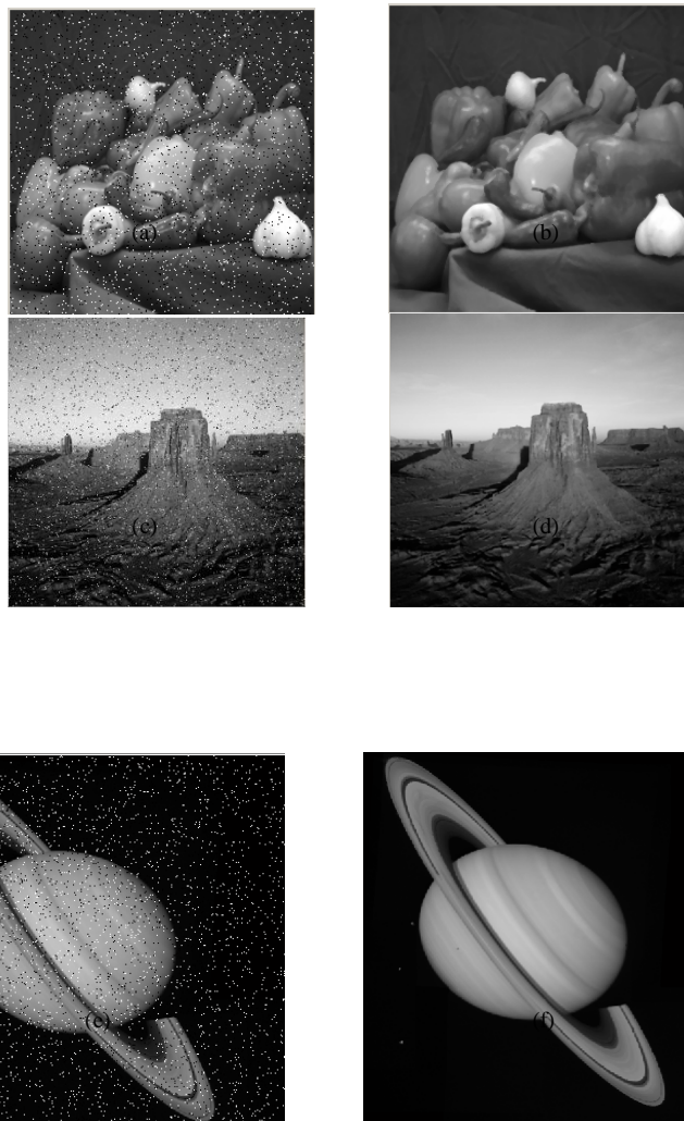
Fig 7. (a) Noisy peppers image, (b) filtered peppers image, (c) Noisy desert image, (d) Filtered desert image, (e) Noisy Saturn image, (f) Filtered Saturn image
