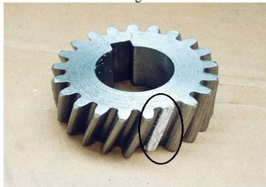
Fig. 3: One tooth missing defect
