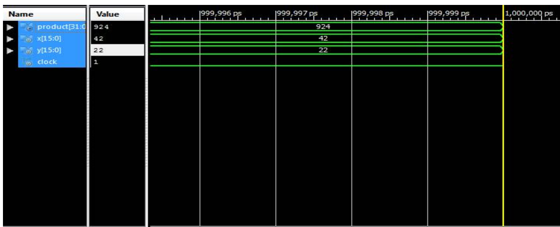
Fig 6:Simulation waveform for 16bit preferred fulladder wallacemultiplier
