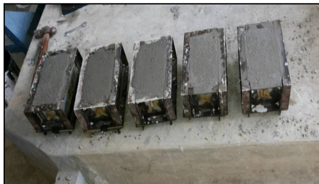
Figure 2. Special moulds with casted concrete blocks
